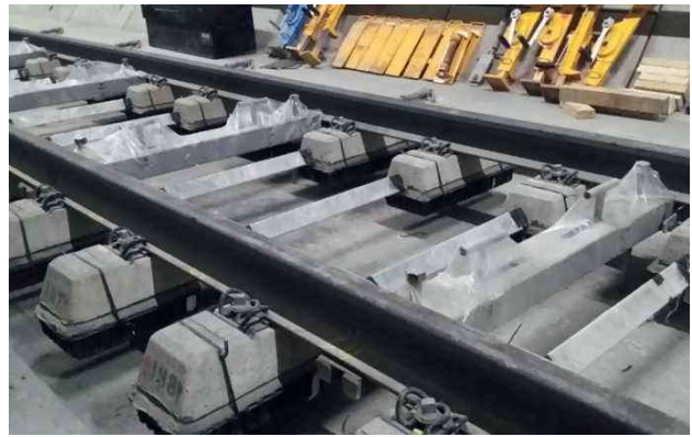
Bi-block sleepers with Sylodyn® insertion pads for sleeper boots
