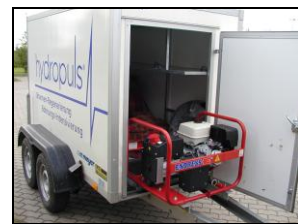
Opened trailer with electro aggregate
